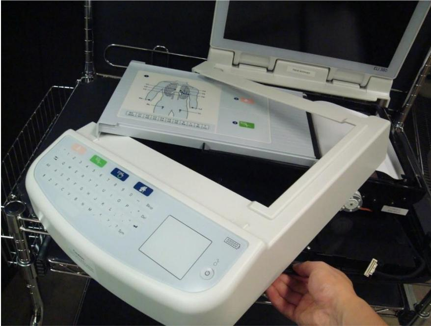
Remove the upper housing assembly and close the writer door.
