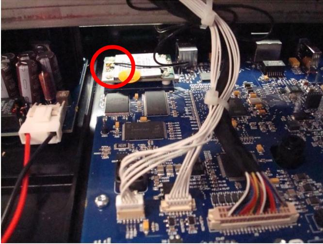
Remove WLAN antenna (Item 13a shown) from the display bracket if replacing the display assembly.
