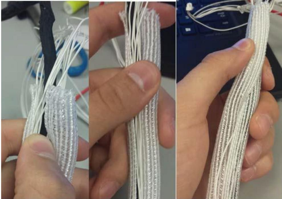
Thread the white display cables through first, and then thread the LVDS cable. You may have to twist the loom to fit it through hinge. If you do, straighten it out before continuing. The loom should be tight inside the hinge and should not move easily.
