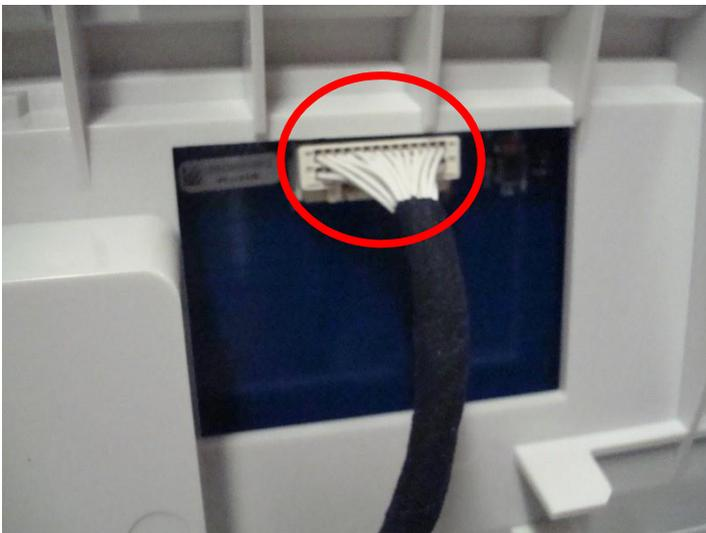
With the keypad cable removed, tilt the lower housing up and slide the upper housing over the extended writer door.
