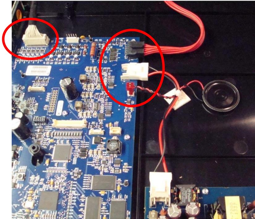
Remove the UTK (Item 35) prior to PCBA removal to avoid damaging the connector.
