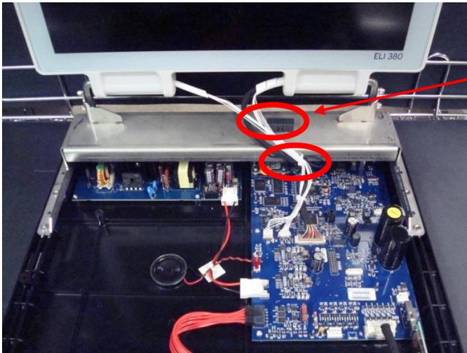
Gently pull straight up on the antenna assembly to remove it from the bracket.
