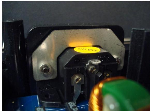
Remove the 2 longer screws (Item 26) holding down the AC input connector, then remove the remaining 3 screws (Item 37) from the PCBA.
