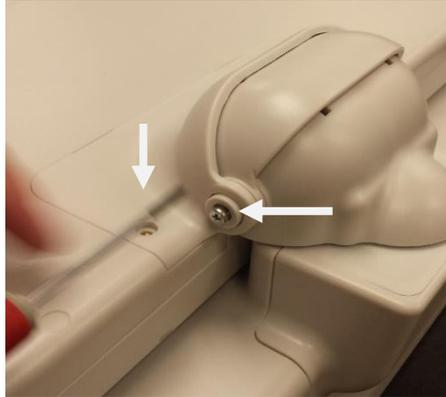
Remove the LCD hinge cover.
