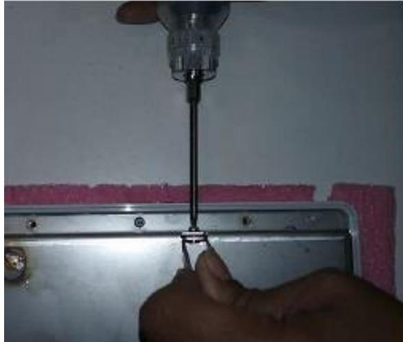
When installing a new LCD Panel Bracket, new cable tie mounts (item 40) will need to be placed directly below the LVDS cable connection as shown below left. To fasten the LCD cables to the mounts, start by bending the LVDS cable to the right of the mounts as shown below right, then secure the LVDS cable to the mount on the right side with a tie wrap (item 16) maintaining a bend so no strain will be applied to the connector end.
