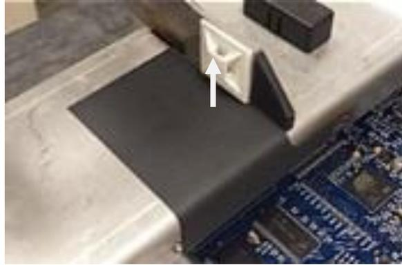
Remove the formex insulator, be sure to clean any residue left over by the formex insulator.
