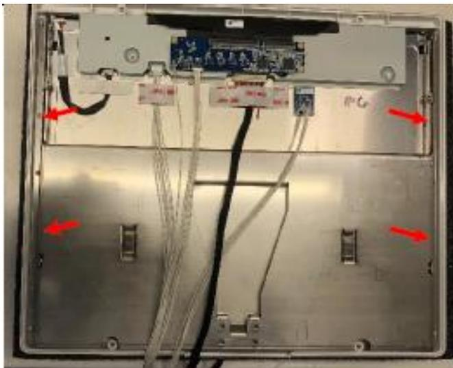
The LCD Panel Bracket is also fastened to the LCD and Bezel assembly by 4 M3x5 screws (6020-530-02) to a torque of 3.5 in/lbs, as shown left below. Remove these 4 screws to lift out the LCD Panel Bracket if replacement is needed.
