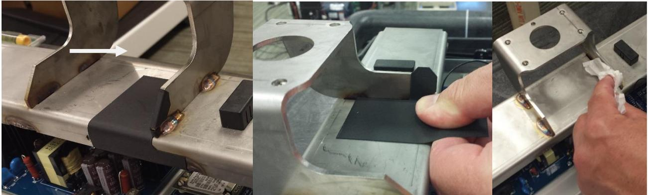
Disconnect the WLAN antenna from ANT2 on the WLAN module. Then remove the WLAN antenna from the metal bracket. Lastly, remove the adhesive kit from the metal bracket (pictures show the B&B WLAN antenna, use similar removal process for the Laird WLAN antenna, items 13b and 61).
