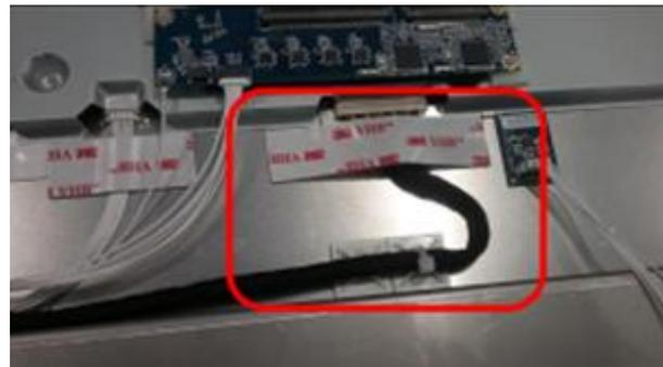
To fasten the remaining cables, apply a similar strain relief bend to the right as shown below, then fasten all 4 cables to the left side mount with a tie wrap (item 16).
