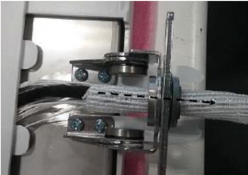
Pull the braided loom past the hinge screws as shown below.
