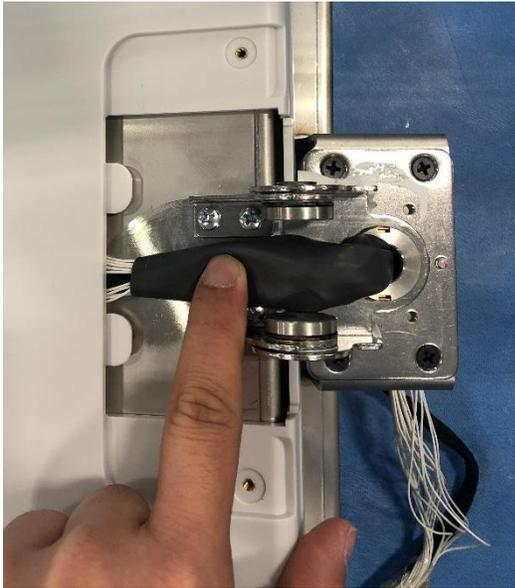
Tighten two cable ties on the Heat Shrink Tubing in opposite direction with a cable tie tool to limit its vertical movement.
