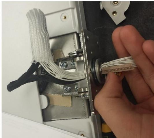
Once the cables are out of the way. Remove the 4 screws from the hinge and hinge cover set.
