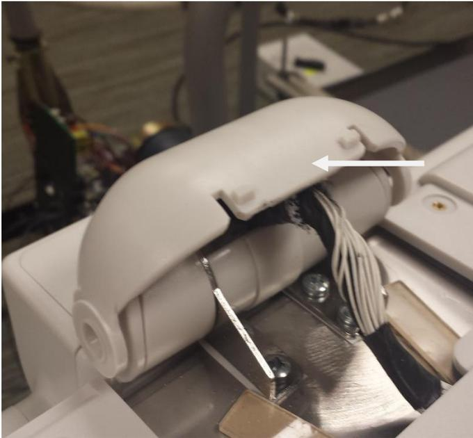
Remove the rear hinge cover vertically.
