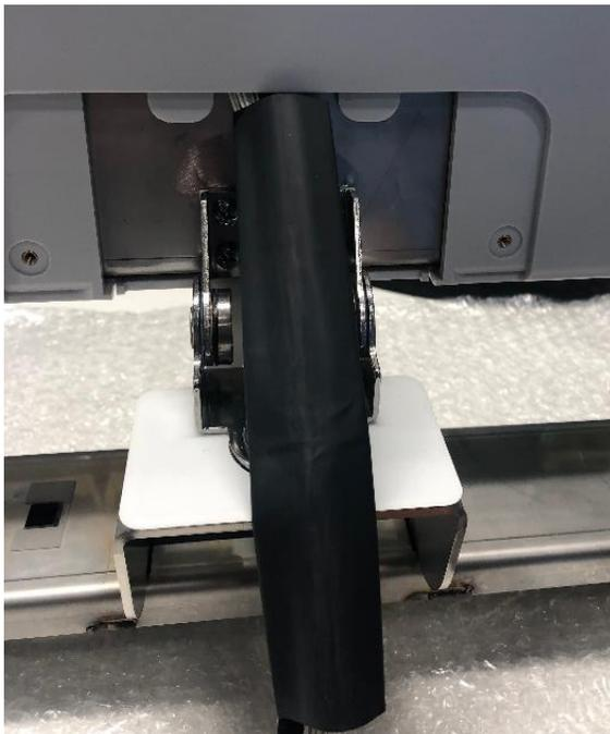
Using a heat shrink gun, apply heat on the heat shrink tubing to snugly wrap the cables.
