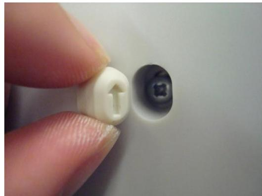
Pull the housing rear cover (Item 29) straight out from the back of the device.
