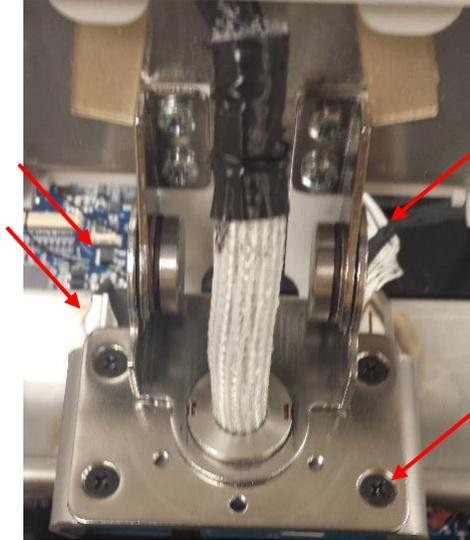
Unthread the cables back through the bracket and hinge.
