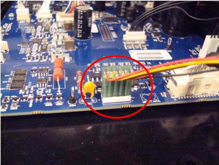
Continue to lift the writer assembly and remove the remaining cable assemblies from the PCBA.
