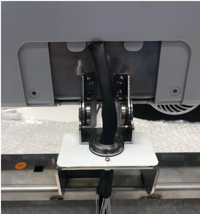
Close the screen, press the Heat Shrink Tubing with cables to make sure it touches the back of the LCD screen. This ensures it has enough slack to open/close the LCD screen.
