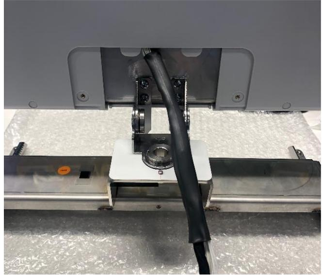
Verify the heat shrink tubing is shrunk adequately round and there is no damage to the cables and LCD back cover due to heat.
