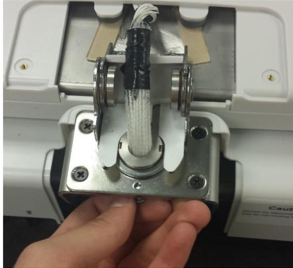
Rotate the screen so that it is facing away from the user side, then remove the rear cover.
