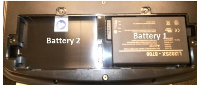
The battery date code is stamped on the side of the battery pack (first 6 digits of string, see picture). Date code for this battery is 131126 (format = YYMMDD).
