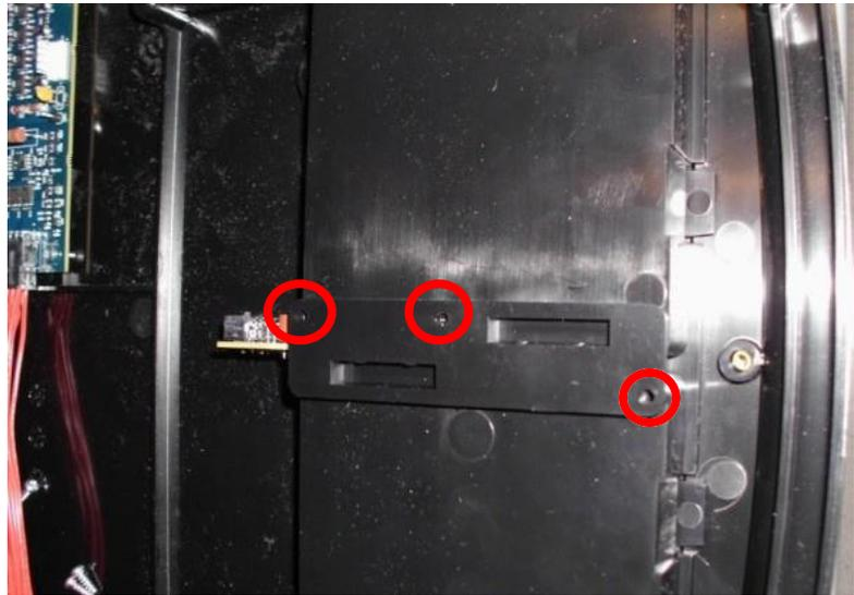
Remove the battery connector board (Item 8) by pulling it straight up from the lower housing.
