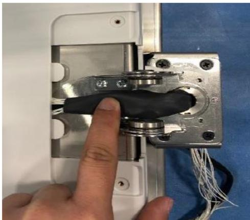
Tighten the four cable ties on the Heat Shrink Tubing in opposite direction to limit its vertical movement (as shown below).
