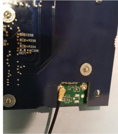
One of two different Laird antenna configurations will be present (item 13b or 13c). The earlier version b antenna has 2 antenna connectors as shown above, the newer version c has only 1 antenna connection.
