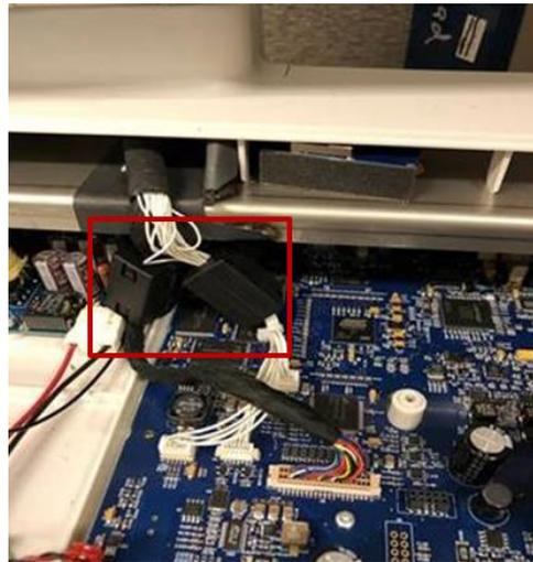
Depending on the age of the unit, it may have 2 display insulators (item 62) as shown below. The insulators were introduced on units built from mid-2019 forward to comply with 4<sup>th</sup> Edition EMC standards. If present, inspect the insulators for signs of wear or damage, and replace if necessary. If the unit did not have the insulators installed, they do not need to be added retrospectively.
