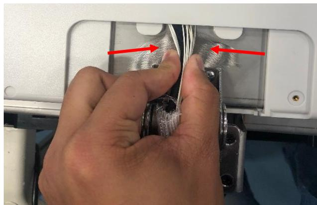
Once verified correct, tighten two cable ties (item #7495-001) to the braided loom in opposite direction to limit its vertical movement.
