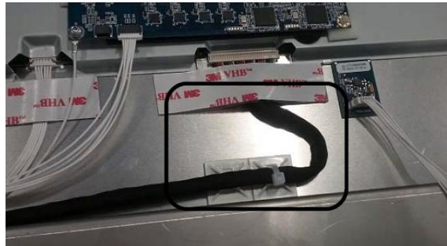
Remove the Acrylic tape (7401-005) holding the cables to the LCD assembly if replacing the associated cable.
