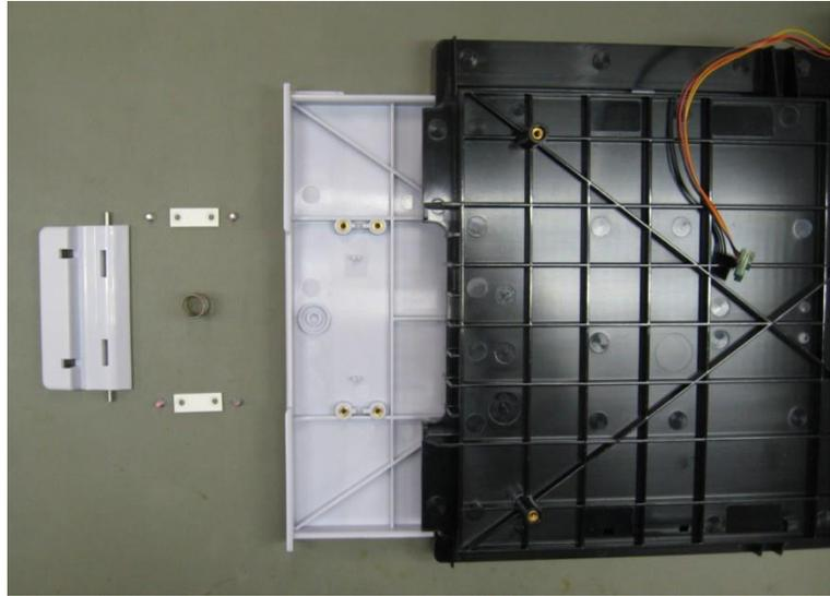
On the other end of the writer assembly, the print head assembly must be removed from its installed position. This is done by removing the O-Ring that holds the assembly in place (underside of area circled) and unlatching the spring bar retaining clips as shown below.
