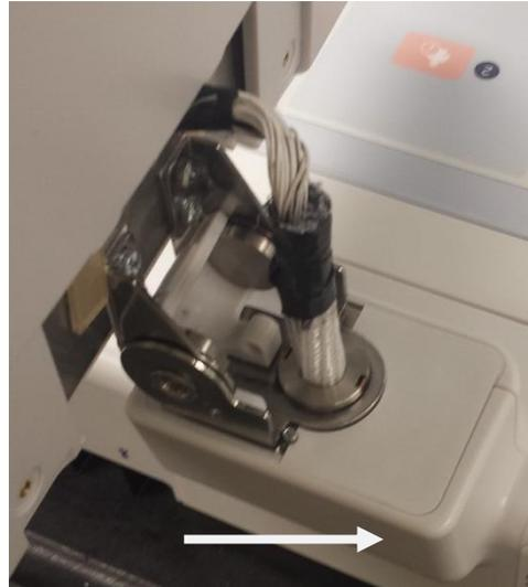
Remove Silicon Plug from the Rear Housing location (item 32).
