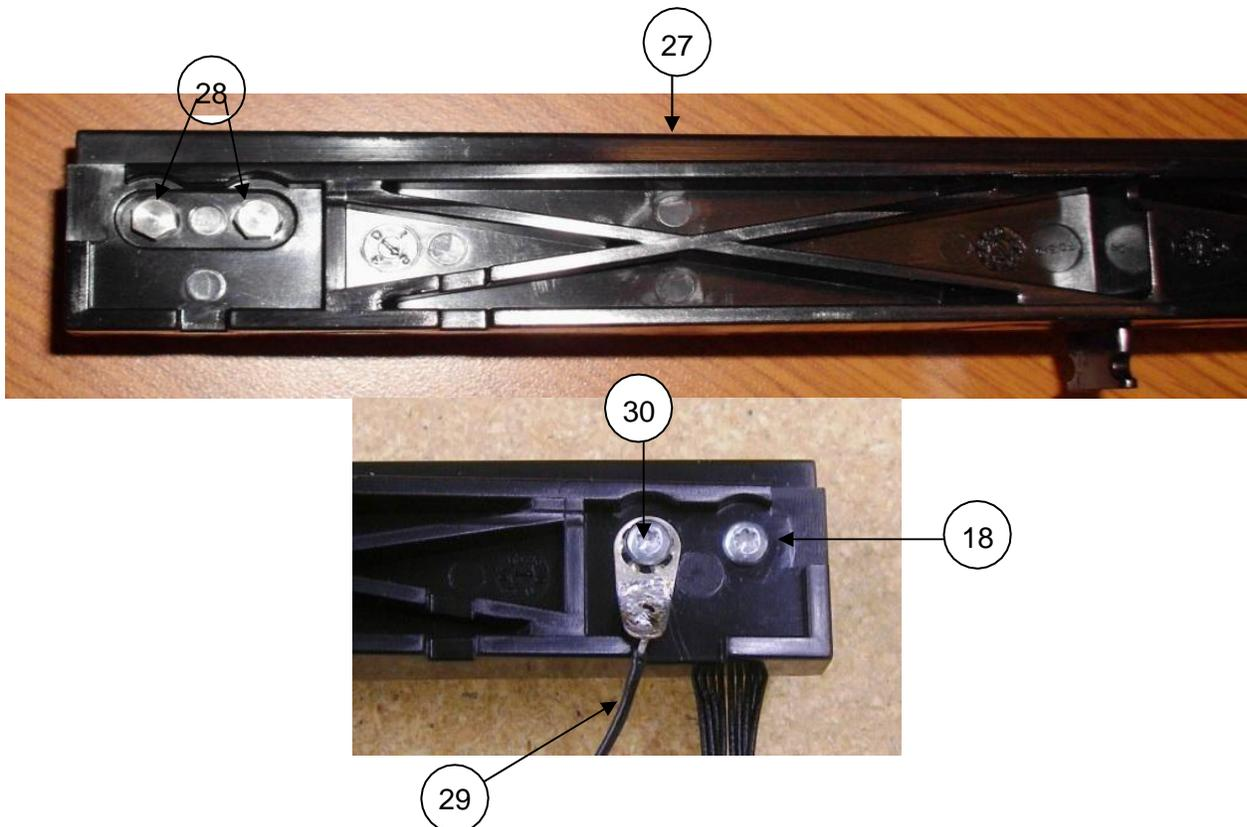
When reinstalling the print head assembly, create a loop with the ground wire to allow it to move freely within the provided slot.
