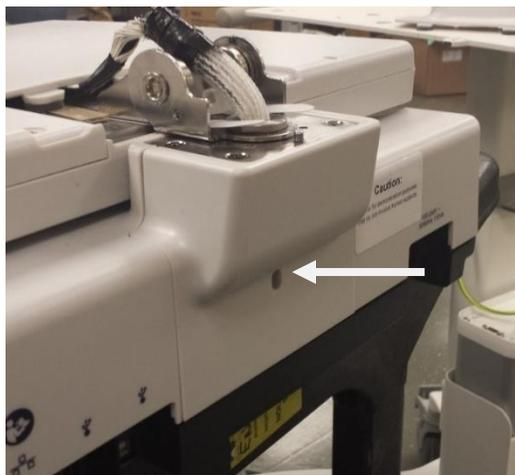
Remove the screw used as the horizontal hinge stop
