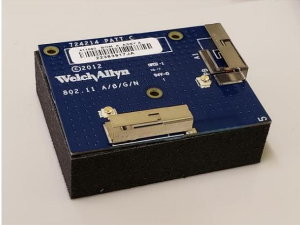
Antenna connection to WLAN module
