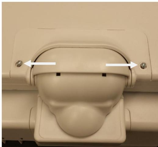
Remove the hinge axel and hinge cover screws from each side of the display as shown below.
