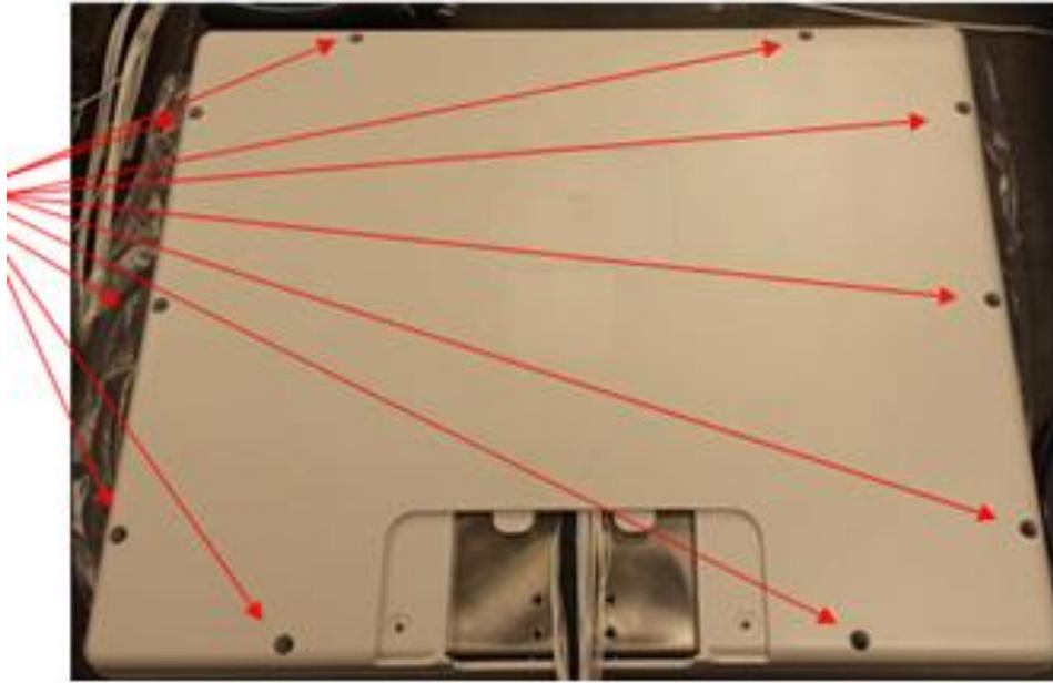
Once the housing screws are removed, clip the cable ties holding the white cables and the LVDS cable as needed.
