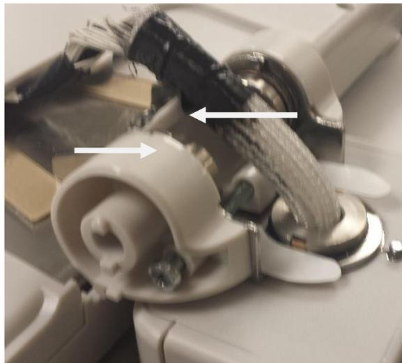
Rotate the screen 90 degrees from user side to remove hinge base sticker. Repeat for other side.
