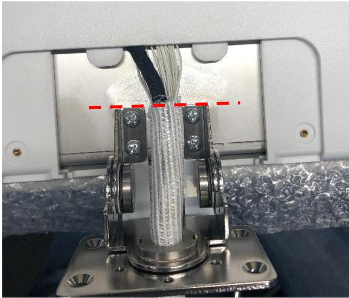
Close the screen, press the cables to make sure it touches the back of the LCD screen. This ensures it has enough slack to open/close the LCD screen.
