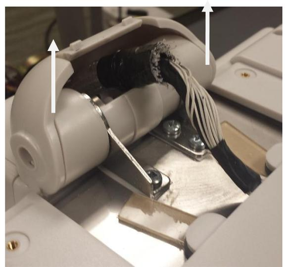
Remove the M4x70 screw from the pivot blocks, then remove the pivot blocks (one from each side).
