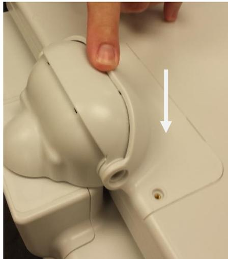
Remove the hinge shutter as shown right.
