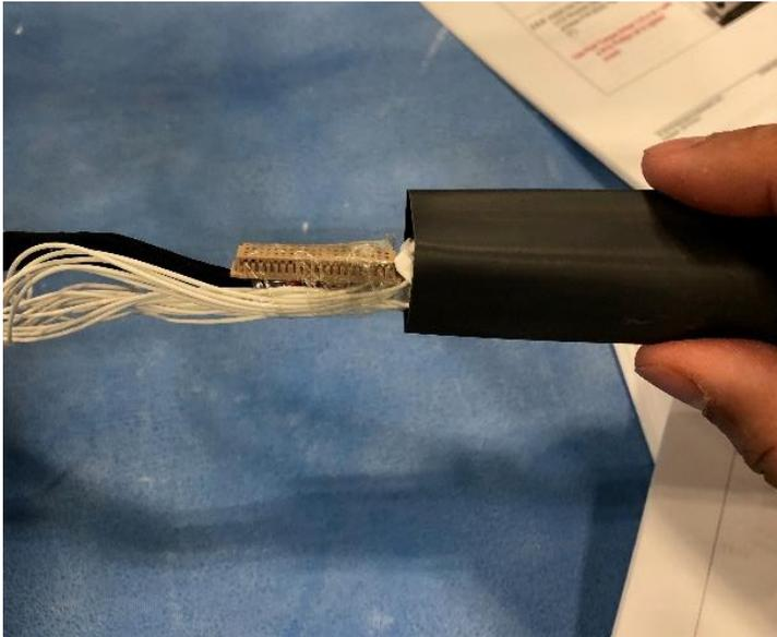
Push the Heat Shrink Tubing upward until it is touching the LCD back cover as shown.
