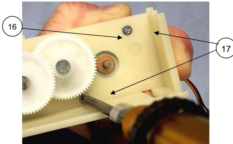
Remove the set screw (9), to remove the stepper motor (15).
