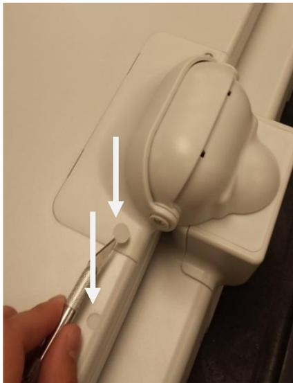
Remove the 2 screws from the LCD hinge.
