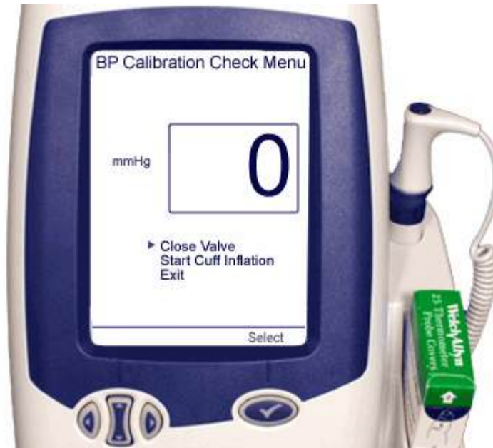
Figure 17. Test Calibration with Closed Valve
