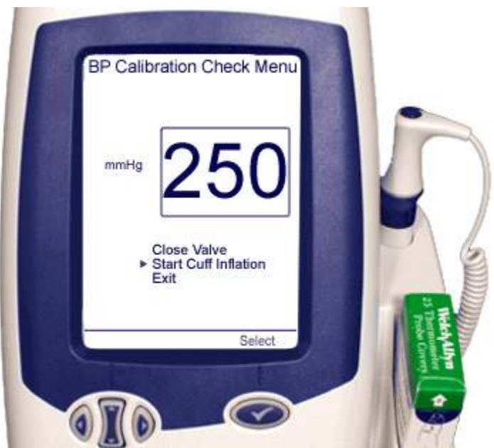
Figure 19. Fine Tune the Pressure Reading to 250 mmHg
