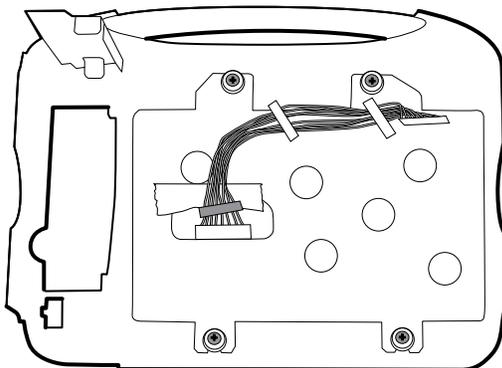
3. Remove the four shoulder screws that secure the LCD frame.
