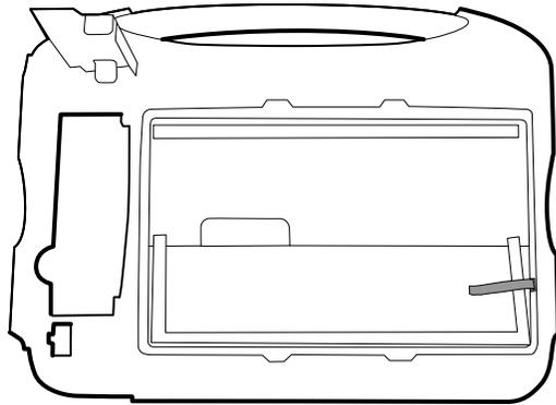
Place the LCD frame over the display. Verify that the LCD frame does not cover the LCD flex cable.
