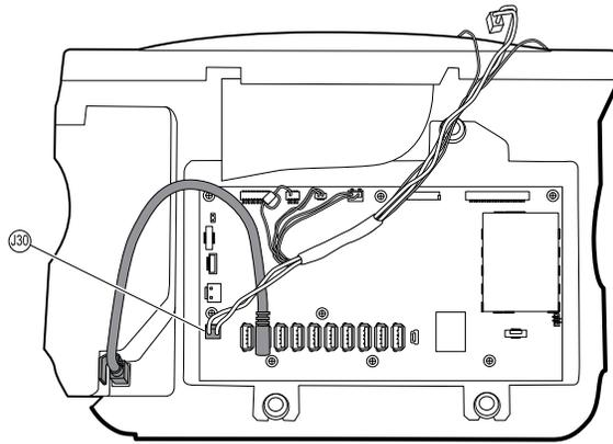
3. Lay the main harness over the top of the unit to clear the USB cables.
