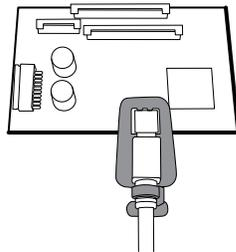
6. Disconnect the USB cables from the main board.
