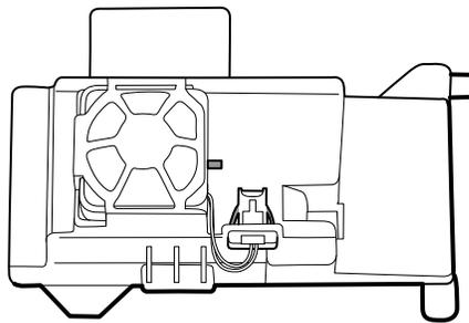
3. Depress the tab on the power-supply cover and slide the fan (19) over the tab and out of the housing.
