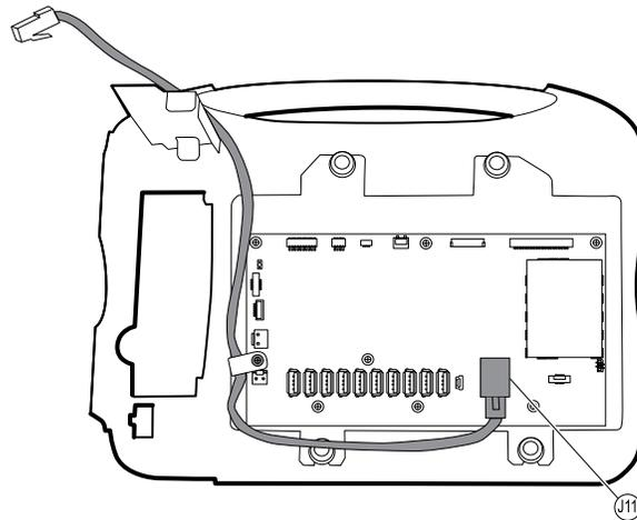
4. Remove the seven screws that secure the main board to the LCD frame.
