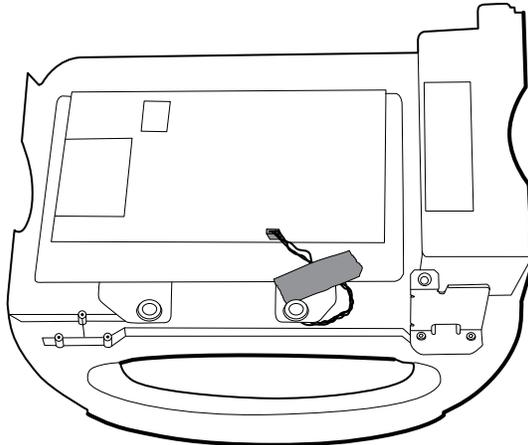
5. Disconnect the light-bar harness from J46 on the main board.
