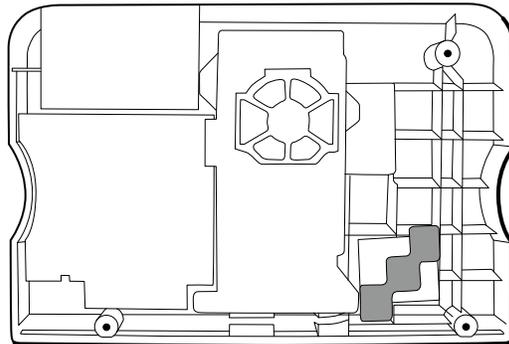
4. Expose the adhesive on the foam block. Mount the antenna (16) on the foam block with the antenna cable (39) oriented under the board and in the wire channel above the power supply.
