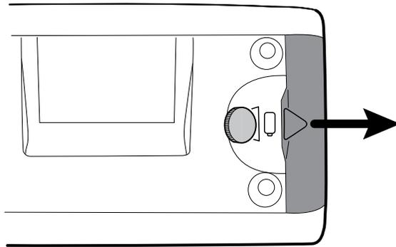
4. Pull the battery out by pulling the battery label, which is visible when you open the battery cover.
