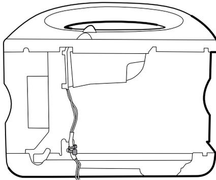
5. Disconnect the speaker cable on the speaker (26) from the main harness.
