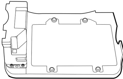
6. Remove the two screws (10) that secure the top of the temperature module.
